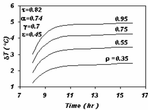
Fig. 11-Effects of mirror reflectivity on the oil temperature
