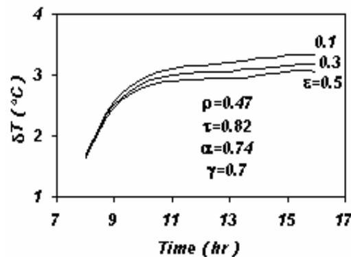
Fig. 9-Effects of tube emissivity on the oil temperature
