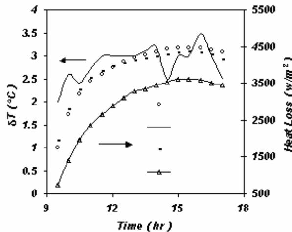
**Fig. 7- Oil temperature difference between outlet and inlet of the receiver (D=Daneshyar model, E=experimental, N=numerical method)**
