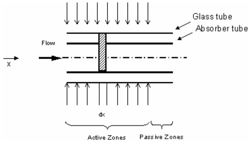
Fig. 4- A section of the receiver tube
