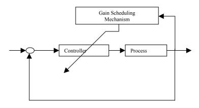
Figure 1- Configuration of Gain Scheduling Controller
