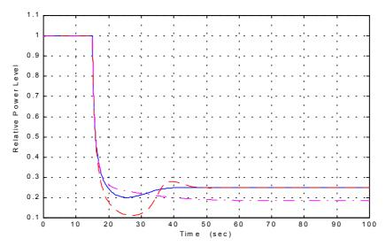
Figure 3- Emergency operation 100% to 25% power level Change
